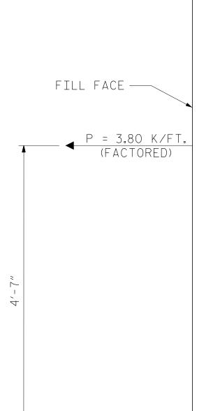
TIE BACK D (DETAIL SHOWING TIE BACK RES FOR MSE RETAINING WALLS, SEE GEOT
