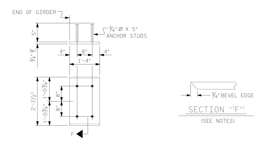
EMBEDDED PLATE "B-1" DETAILS TWO EMBEDDED PLATES "B-1" ARE REQUIRED FOR EACH GIRDER.
