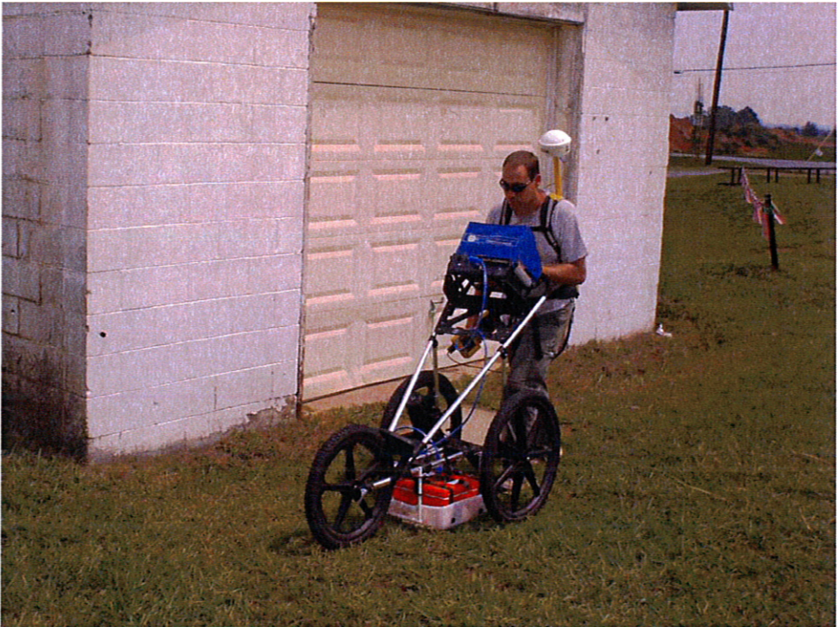
Geophysical Survey Systems SIR-3000 with 400 MHz antenna
