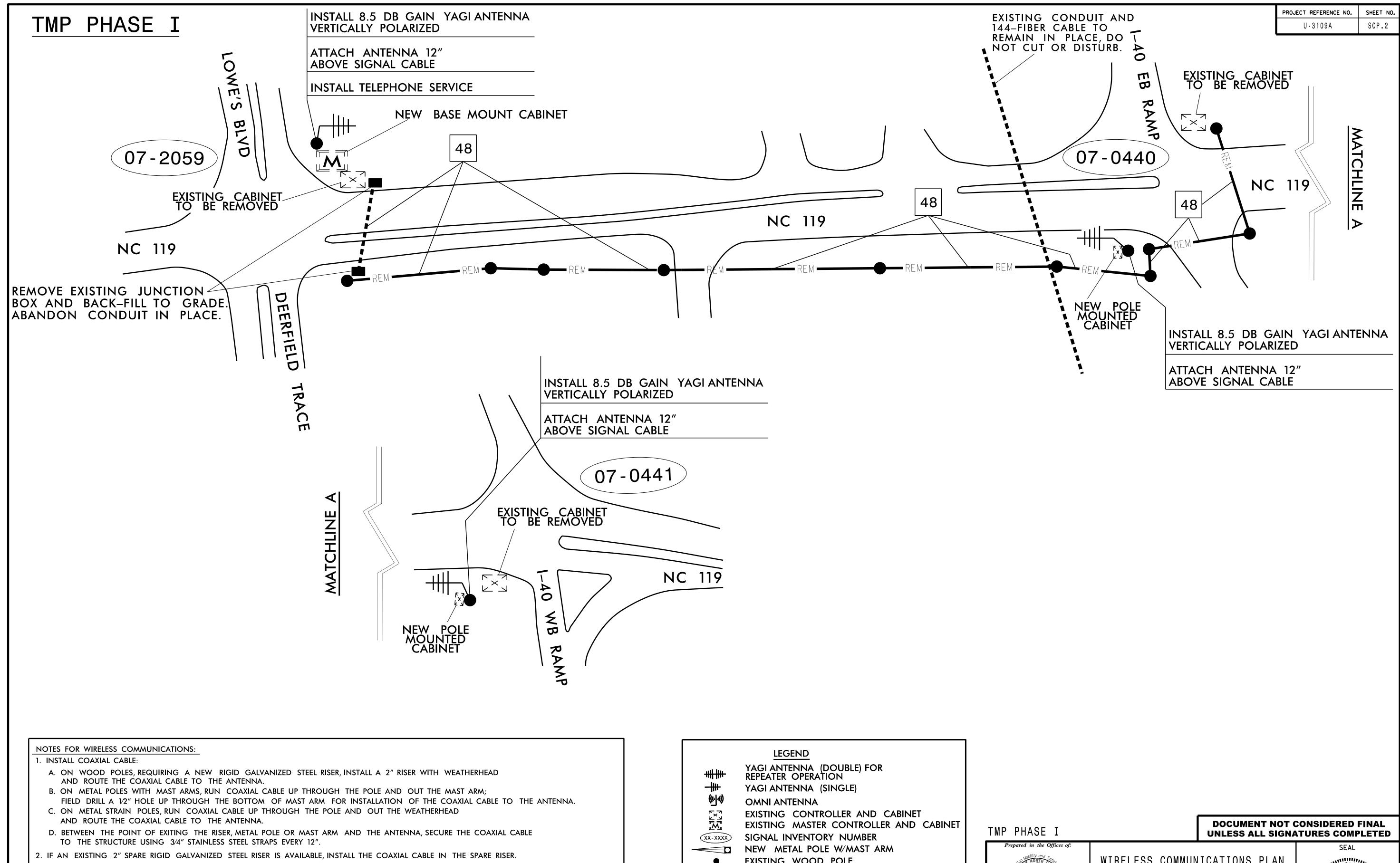
3. INSTALL WIRELESS ANTENNA ON POLE WITH RF WARNING SIGN. (NOTE: RF WARNING SIGN NOT REQUIRED WHEN ANTENNA IS INSTALLED ON AN NCDOT-OWNED POLE.) 4. MAINTAIN PROPER CLEARANCE FROM ALL UTILITIES PER THE NATIONAL ELECTRICAL SAFETY CODE. 5. INSTALL WIRELESS SERIAL RADIO MODEM WITH EXTERIOR DISCONNECT SWITCH LOCATED ON CABINET. (NOTE: RF ANTENNA DISCONNECT SWITCH AND DECAL ARE NOT REQUIRED WHEN THE ANTENNA IS INSTALLED ON AN NCDOT-OWNED POLE.)
