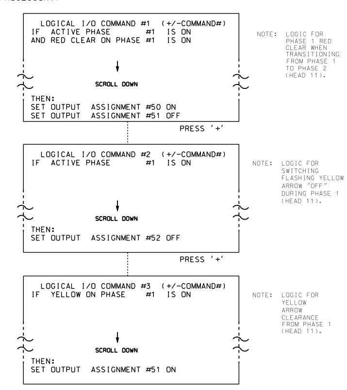
LOGIC I/O PROCESSOR PROGRAMMING COMPLETE
