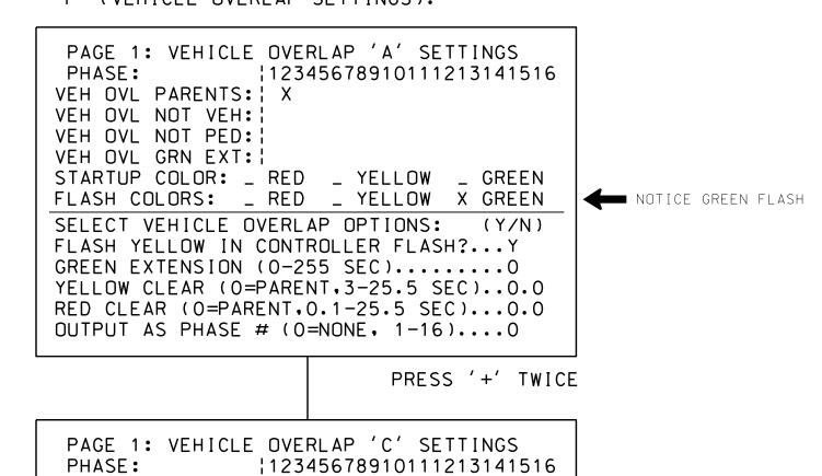
VEH OVL PARENTS: | XX VEH OVL NOT VEH: VEH OVL NOT PED: | VEH OVL GRN EXT: | STARTUP COLOR: \_ RED \_ YELLOW \_ GREEN FLASH COLORS: \_ RED \_ YELLOW X GREEN NOTICE GREEN FLASH SELECT VEHICLE OVERLAP OPTIONS: (Y/N) FLASH YELLOW IN CONTROLLER FLASH?...Y GREEN EXTENSION (0-255 SEC).....0 YELLOW CLEAR (O=PARENT,3-25.5 SEC)..0.0 RED CLEAR (0=PARENT, 0.1-25.5 SEC)...0.0 OUTPUT AS PHASE # (0=NONE, 1-16)....0
