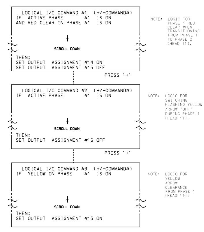
LOGIC I/O PROCESSOR PROGRAMMING COMPLETE
