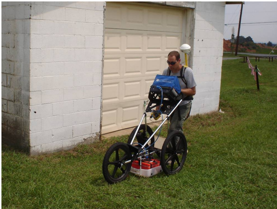
GSSI SIR-3000 Ground-Penetrating Radar with 400 MHz Antenna
