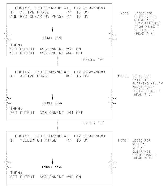
LOGIC I/O PROCESSOR PROGRAMMING COMPLETE
