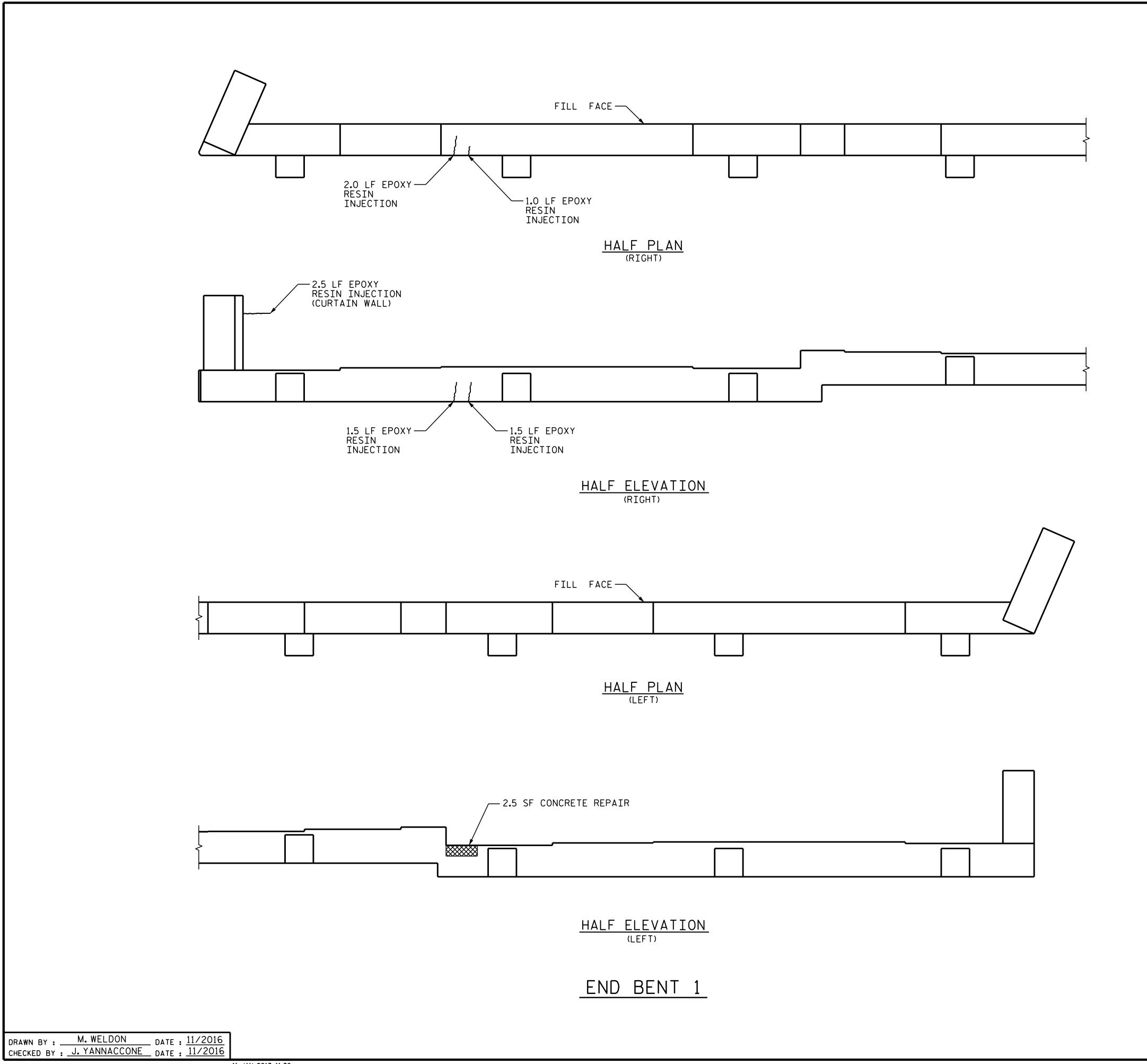
AS-BUILT REPAIR QUANTITY TABLE REPAIRS QUANTITIES END BENT ACTUAL ESTIMATE AREA VOLUME AREA VOLUME SHOTCRETE REPAIRS SF CF 0.0 0.0 CURTAIN WALL 0.0 0.0 AREA VOLUME AREA VOLUME CONCRETE REPAIRS CF CF CAP 2.5 1.2 **\*** EPOXY RESIN INJECTION FΤ 6.0 CAP
