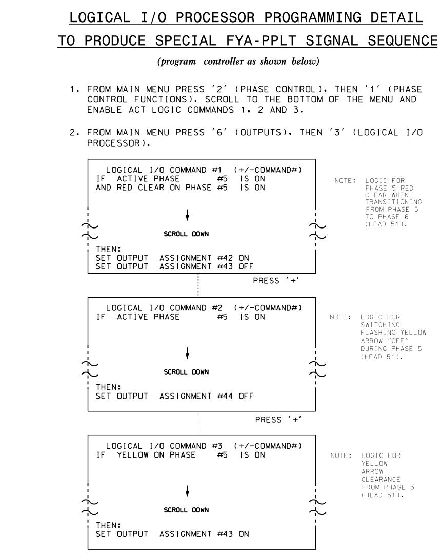
LOGIC I/O PROCESSOR PROGRAMMING COMPLETE
