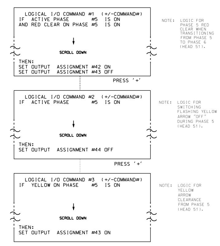
LOGIC I/O PROCESSOR PROGRAMMING COMPLETE
