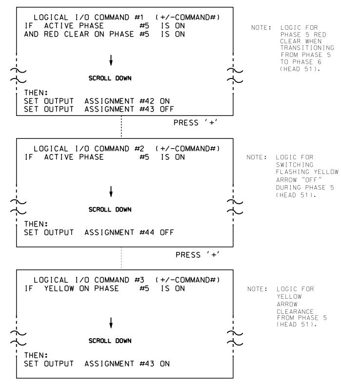
LOGIC I/O PROCESSOR PROGRAMMING COMPLETE
