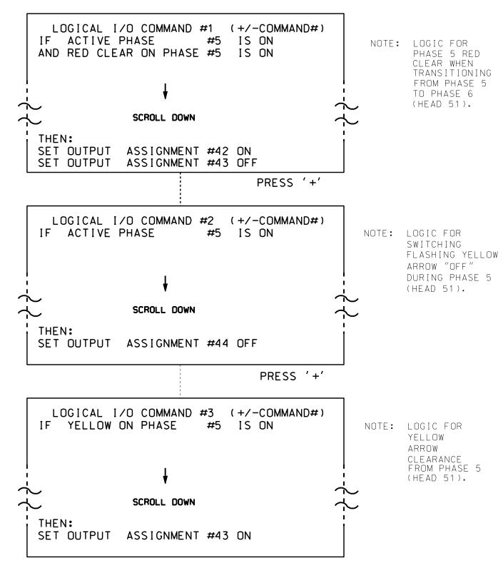
LOGIC I/O PROCESSOR PROGRAMMING COMPLETE
