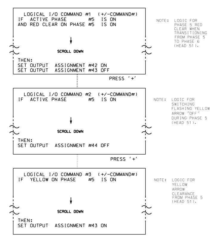
LOGIC I/O PROCESSOR PROGRAMMING COMPLETE
