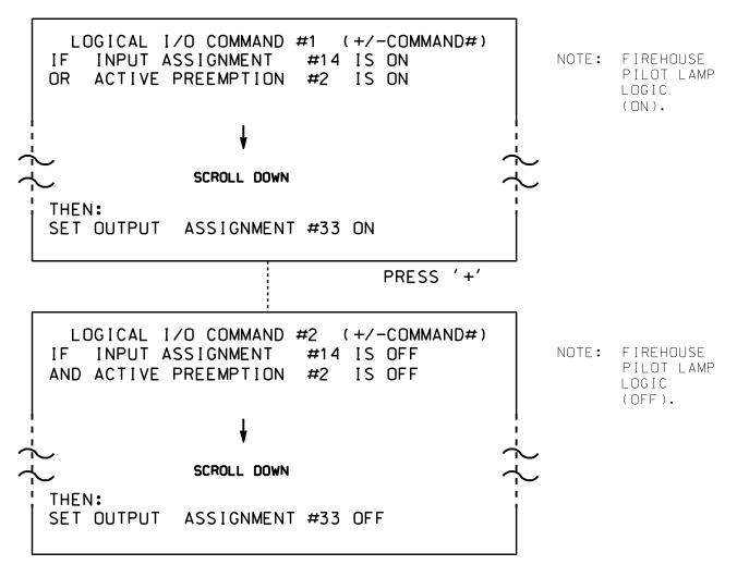
LOGIC I/O PROCESSOR PROGRAMMING COMPLETE
