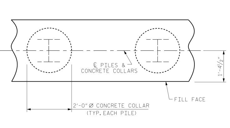
CONCRETE — COLLAR BOTTOM OF CAP © HP 12 X 53 TEEL PILE 2'-0" ELEVATION
