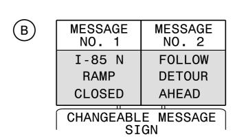
MIN. 350 FT IN ADVANCE OF I-85 N ENTRANCE RAMP OR AS DIRECTED BY ENGINEER MIN. 350 FT IN ADVANCE OF I-85 S ENTRANCE RAMP OR AS DIRECTED BY ENGINEER
