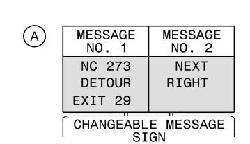
MIN. 1500 FT IN ADVANCE OF EXIT 29 DECELERATION LANE OR AS DIRECTED BY ENGINEER
