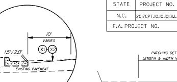
DETAIL FOR PROFILE MILLING (0" TO 1.5") DETAIL FOR PROFILE MILLING (0" TO 2.0")
