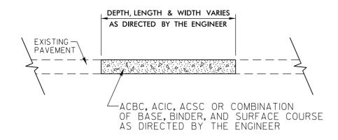
DETAIL FOR PATCHING EXISTING PAVEMENT
