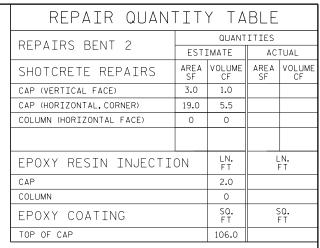
VALUES IN CHART REPRESENT ESTIMATED REPAIR TOTALS AFTER REMOVAL OF UNSOUND CONCRETE, MIN. OF 1"BEHIND REBAR AND MIN. 2"CL TO SAWCUT. SEE REPAIR DETAILS.
