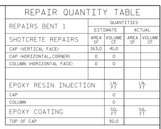
VALUES IN CHART REPRESENT ESTIMATED REPAIR TOTALS AFTER REMOVAL OF UNSOUND CONCRETE, MIN. OF 1"BEHIND REBAR AND MIN. 2"CL TO SAWCUT. SEE REPAIR DETAILS.
