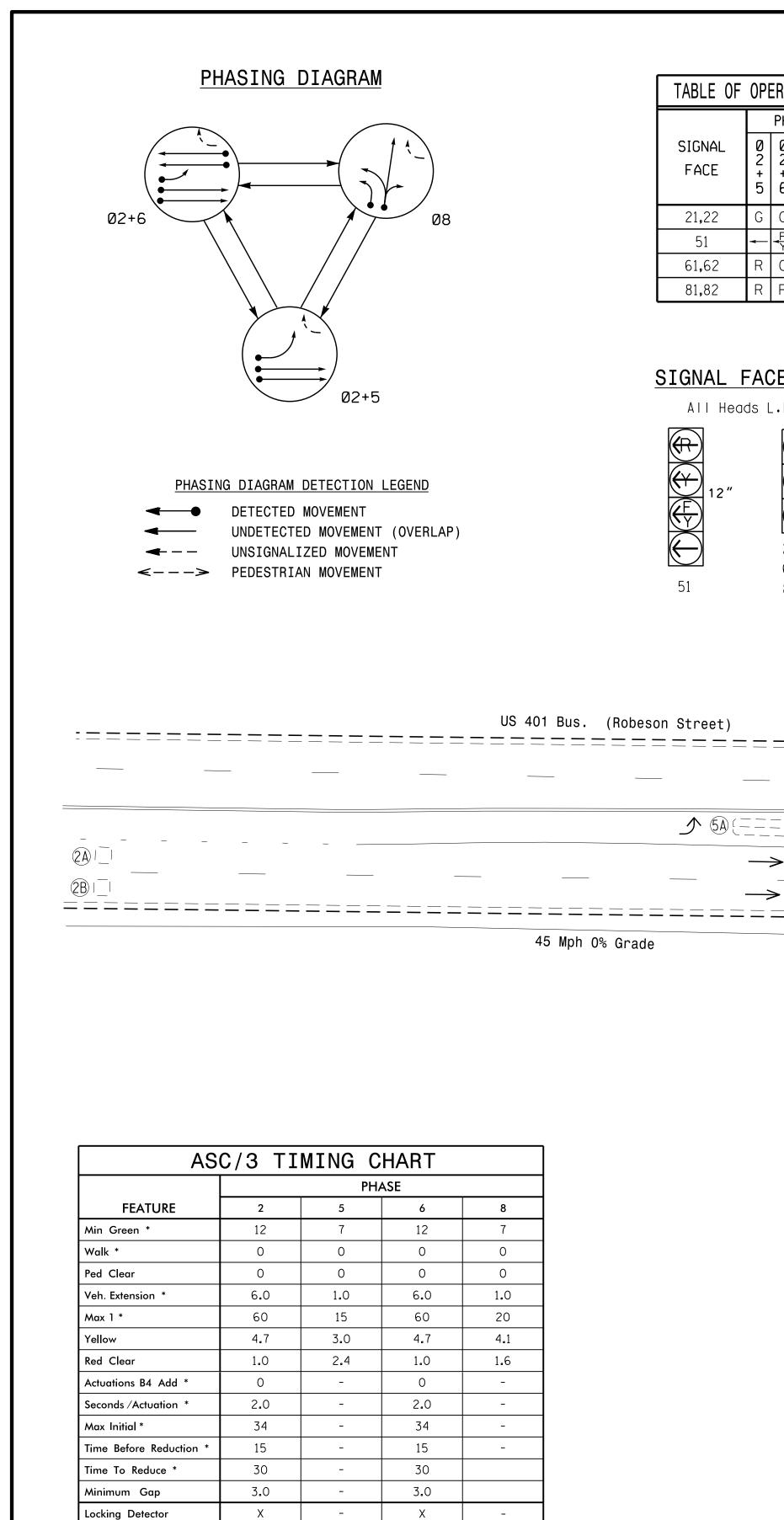
\* These values may be field adjusted. Do not adjust Min Green and Extension times for phases 2 and 6 lower than what is shown. Min Green for all other phases should not be lower than 4 seconds.
