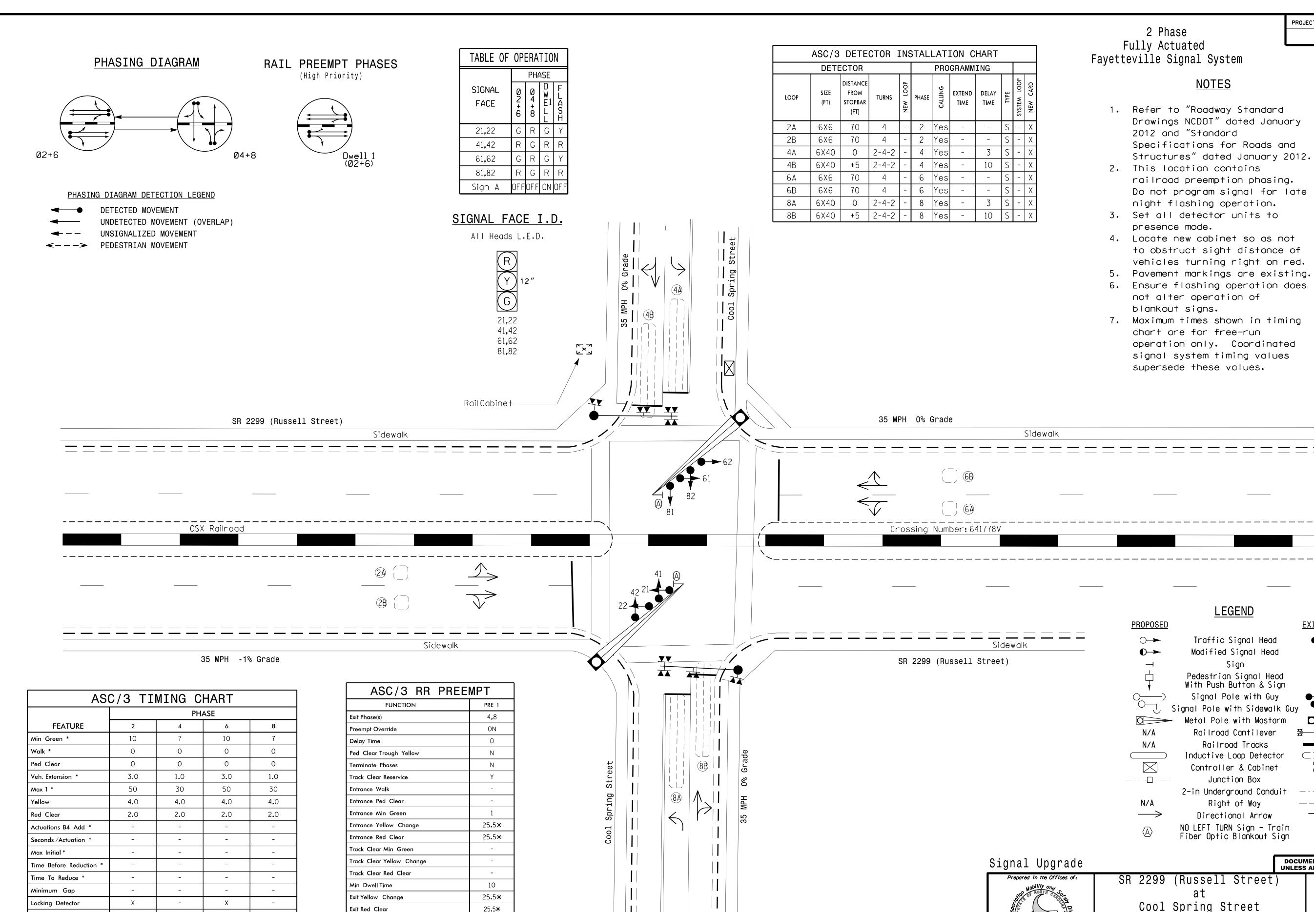
\* These values may be field adjusted. Do not adjust Min Green and Extension times for phases 2 and 6 lower than what is shown. Min Green for all other phases should not be lower than 4 seconds.
