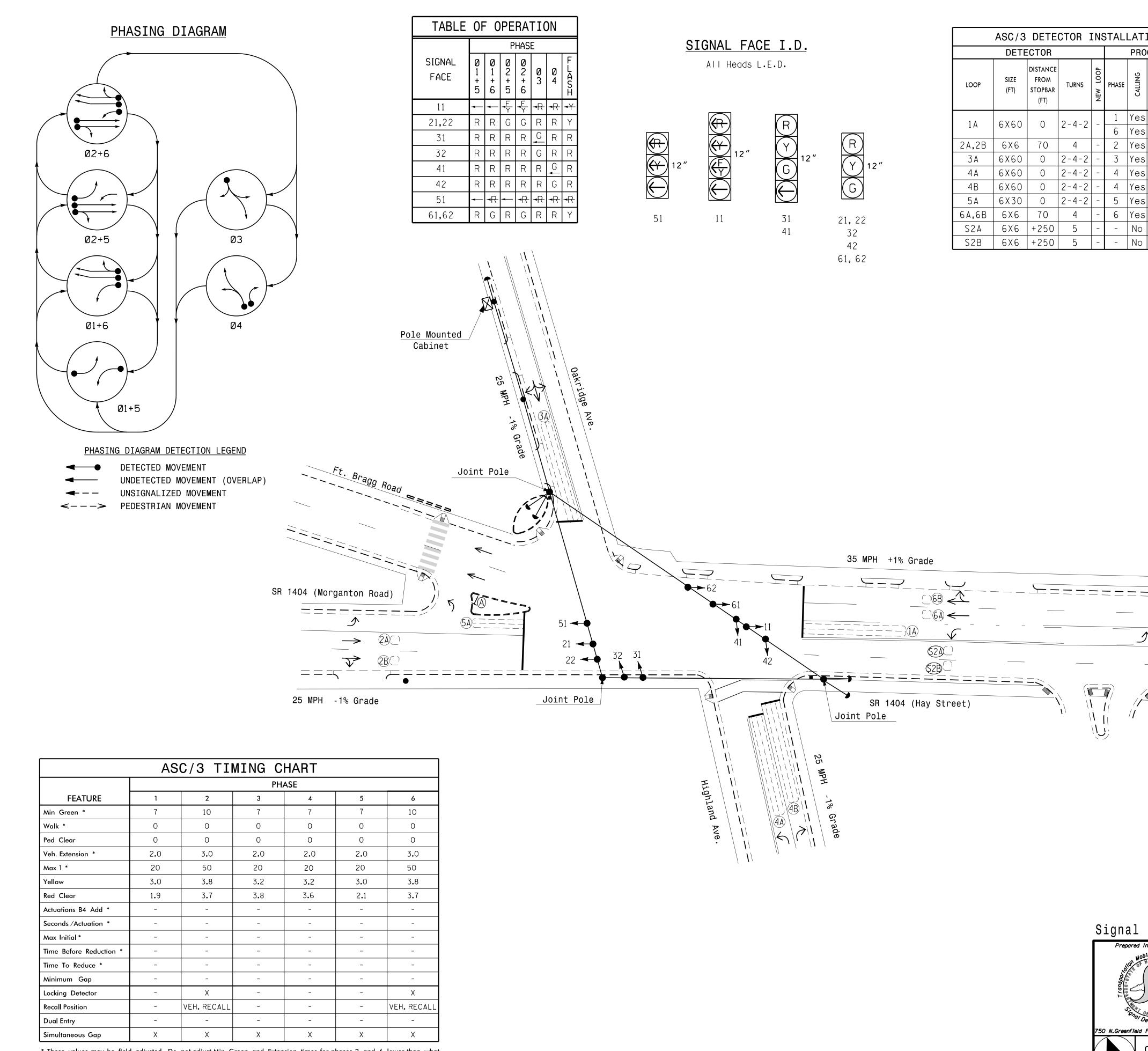
\* These values may be field adjusted. Do not adjust Min Green and Extension times for phases 2 and 6 lower than what is shown. Min Green for all other phases should not be lower than 4 seconds.
