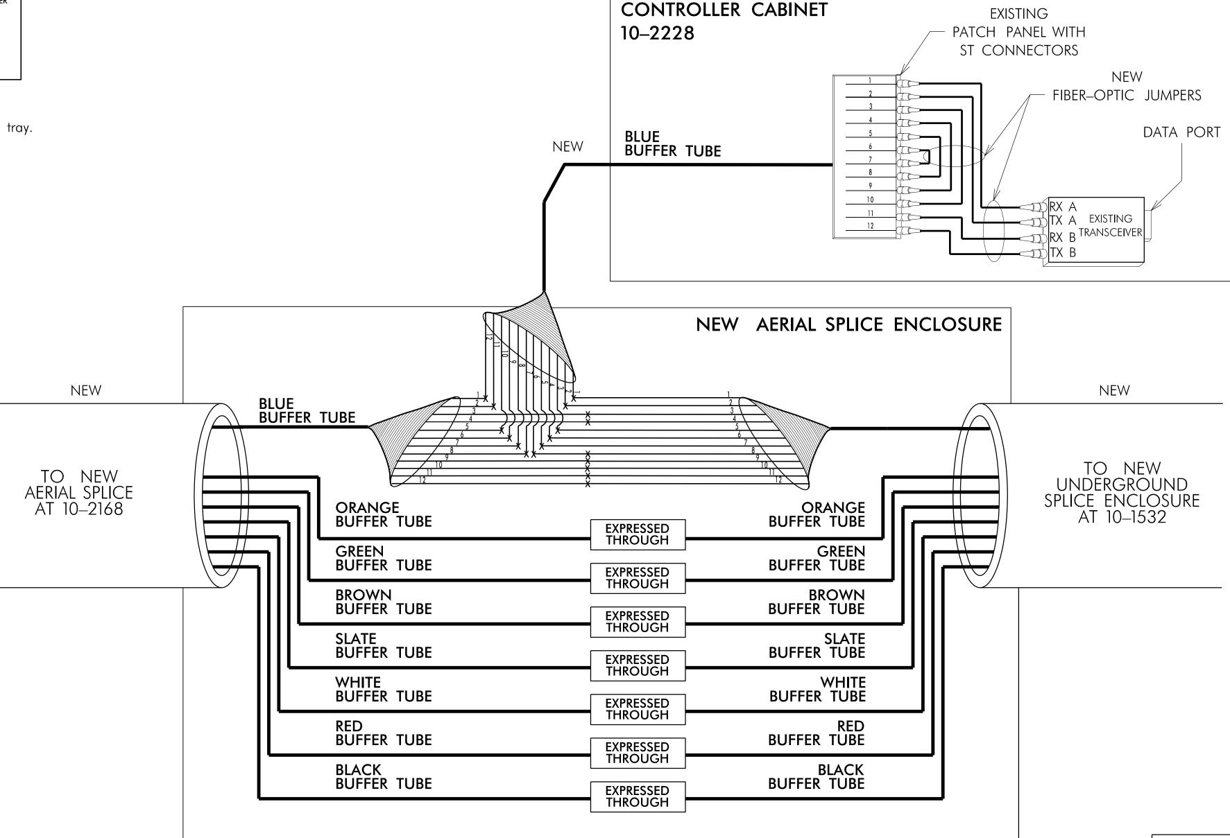
INCLUDE ON THE COVER OF EACH SPLICE TRAY THE FOLLOWING: REFERENCE SECTION 1731 "FIBER OPTIC SPLICE ENCLOSURE"
