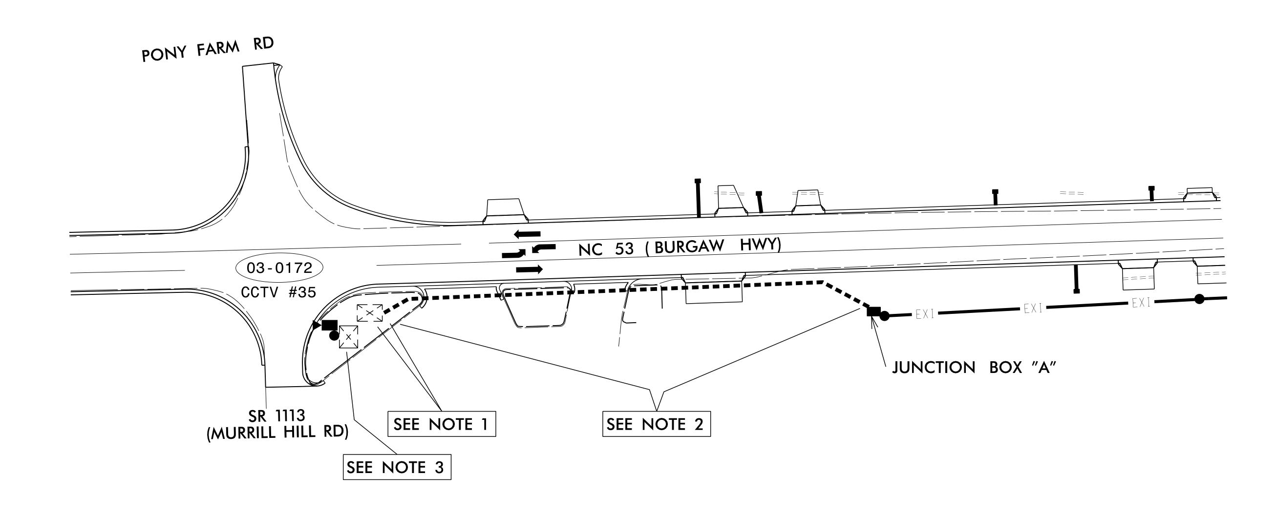
1) CONTRACTOR TO RECORD EXISTING SPLICE ARRANGEMENT FOR COMPARISON TO THE SUPPLIED SPLICE PLANS. IF DISCREPANCIES EXIST, CONTACT THE ENGINEER TO DETERMINE HOW TO PROCEED.
