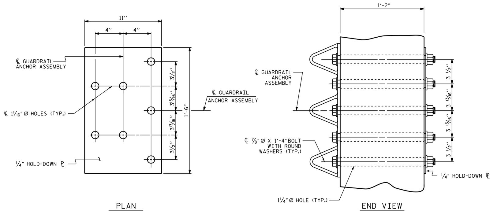
**GUARDRAIL ANCHOR ASSEMBLY DETAILS**
