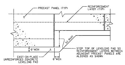
PRECAST CONCRETE PANELS LEVELING PAD STEP DETAIL
