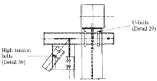
Beam-Column Connection for Truss Structure
