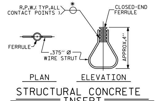
\* EACH WELDED ATTACHMENT OF WIRE TO FERRULE SHALL DEVELOP THE TENSILE STRENGTH OF THE WIRE.
