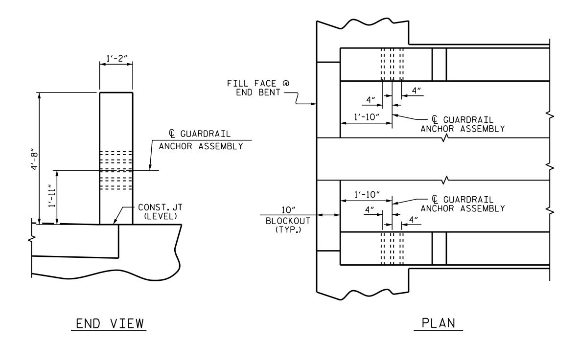
LOCATION OF GUARDRAIL ANCHOR AT END POST
