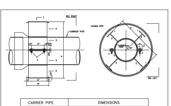
8" x 2" x 1/4" PL 6" x 1 1/2" x 1/4"PL 6" x 1/4"PL 3/8" NUT & BOLT 8" x 3" x 1/4" PL | 6" x 3 1/4" x 1/4"PL | 6" x 1/4"PL | 1/2" NUT & BOLT 8" x 4" x 1/4" PL 6" x 3 5/8" x 3/8"PL 6" x 3/8"PL 1/2" NUT & BOLT 8" x 4" x 3/8" PL 6" x 4 3/4" x 3/8"PL 6" x 3/8"PL 1/2" NUT & BOLT
