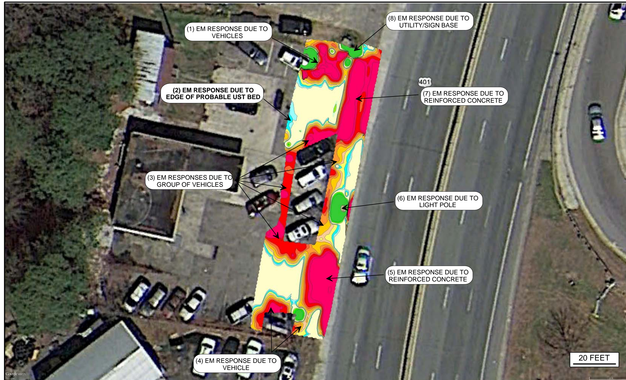
Locations of metallic anomalies detected by the EM61 survey. Numbers correspond to descriptive Table in report.
