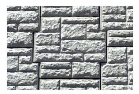
All texture is to be in addition to the nominal thickness of each element within tolerances. Relief of any texture is not to exceed a maximum depth of 1 5/8 inch. The pattern of the form liner must be reviewed and accepted by the Engineer. The Contractor is required to use the same source of form liner for all required elements.
