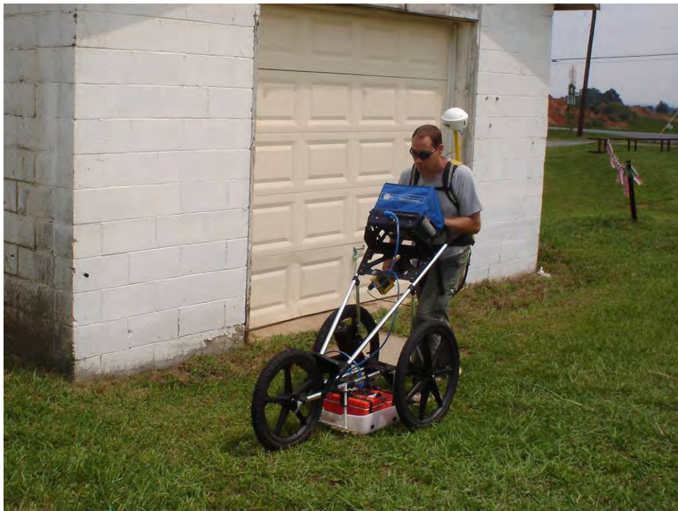
GSSI SIR-3000 Ground-Penetrating Radar with 400 MHz Antenna
