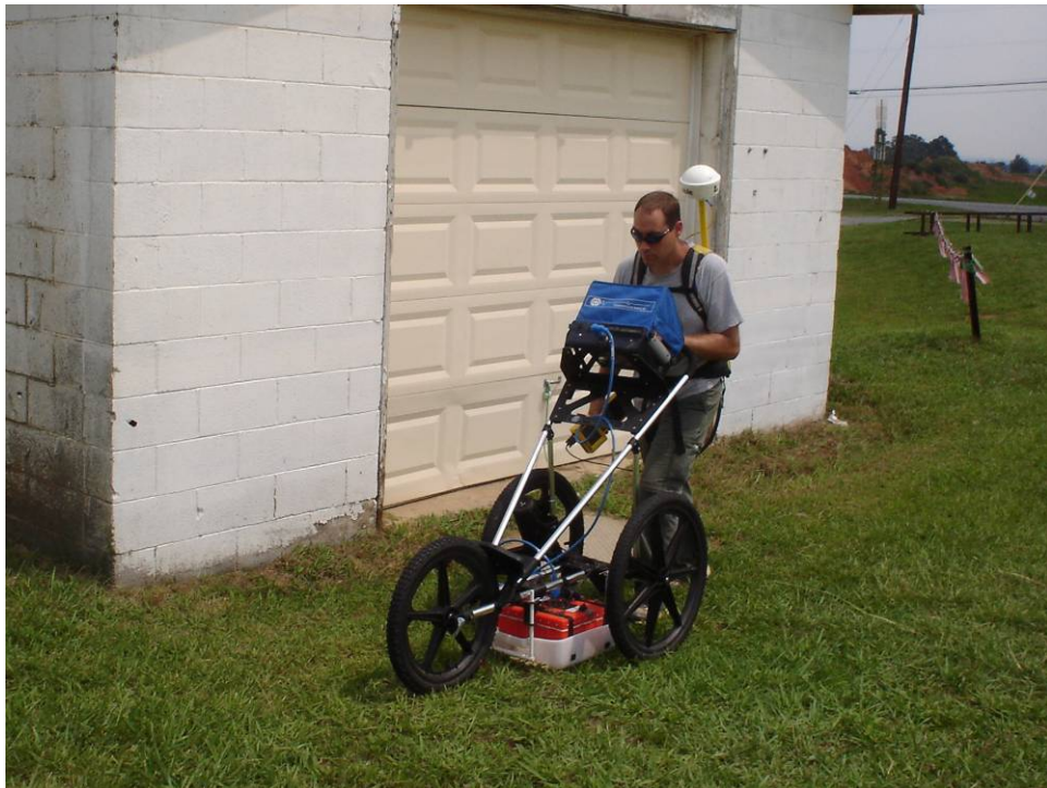
GSSI SIR-3000 Ground-Penetrating Radar with 400 MHz Antenna
