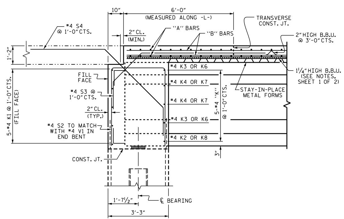
SECTION THROUGH INTEGRAL END BENT
