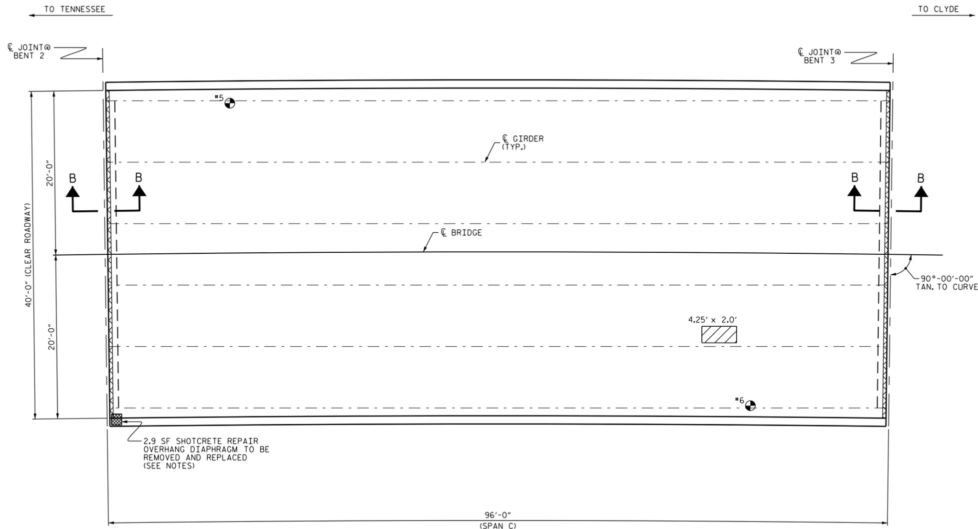
2.9 SF SHOTCRETE REPAIR OVERHANG DIAPHRAGM TO BE REMOVED AND REPLACED (SEE NOTES)
