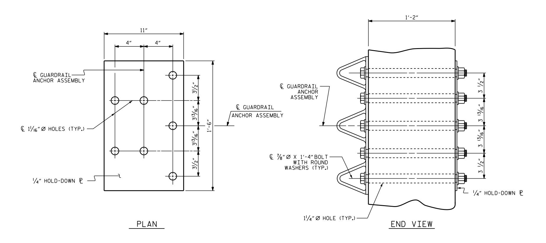
GUARDRAIL ANCHOR ASSEMBLY DETAILS
