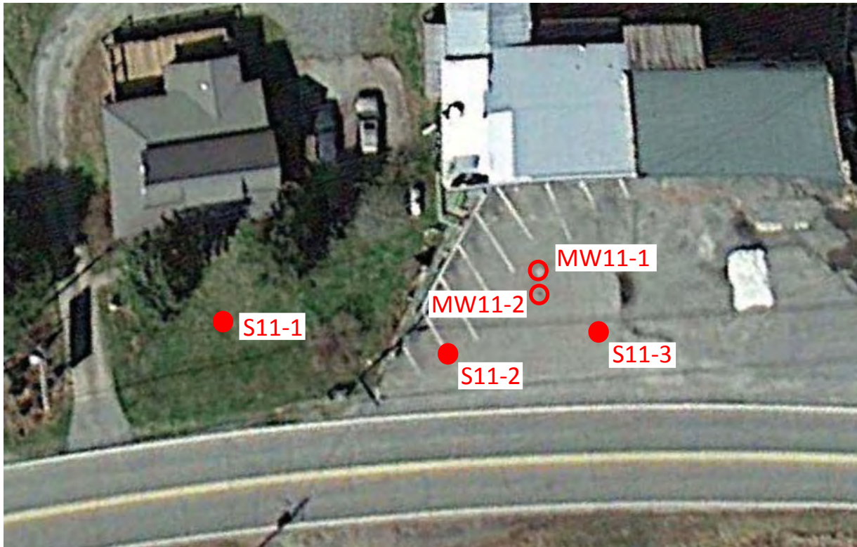
Photograph 1: Aerial view showing boring locations S11-1, S11-2, and S11-3, and existing groundwater monitoring wells MW11-1 and MW11-2 on parcel 011. West is at the top of photo (aerial photo is from Google Earth).
