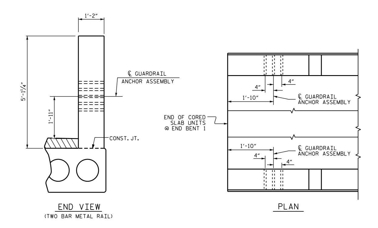
LOCATION OF GUARDRAIL ANCHOR AT END POST
