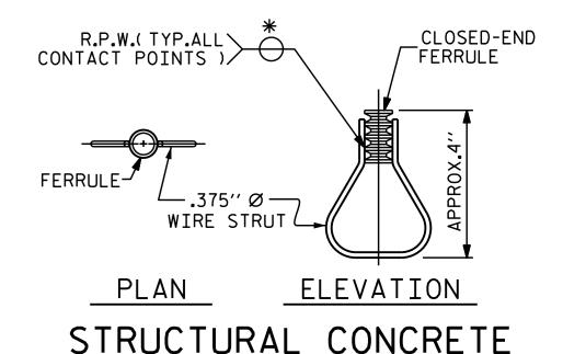
\* EACH WELDED ATTACHMENT OF WIRE TO FERRULE SHALL DEVELOP THE TENSILE STRENGTH OF THE WIRE.
