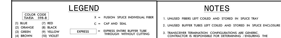
BUFFER SPLICE = SPLICE ALL FIBERS IN BUFFER
