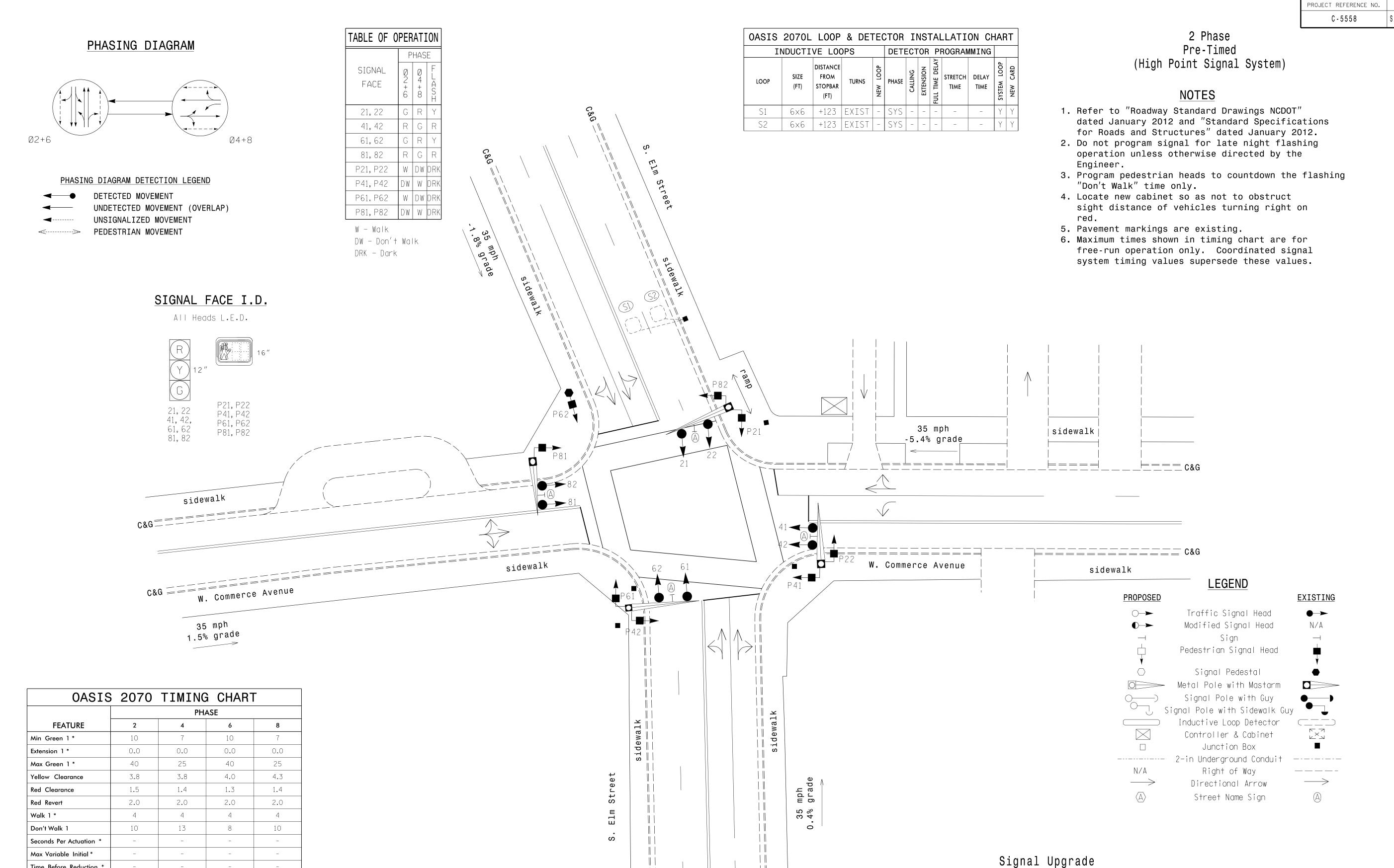
ON \* These values may be field adjusted. Do not adjust Min Green and Extension times for phases 2 and 6 lower than what is shown. Min Green for all other phases should not
