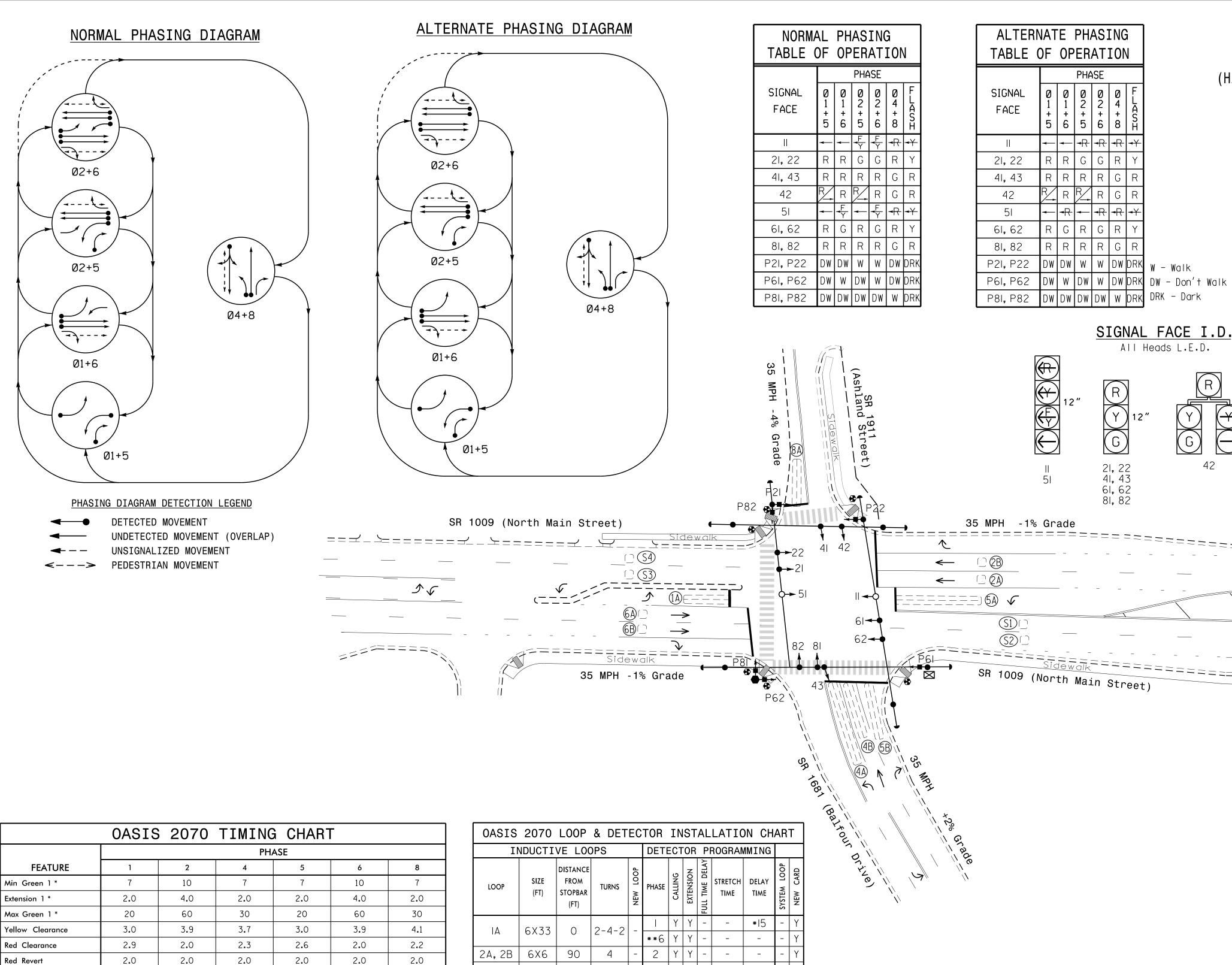
5 Phase Fully Actuated (High Point Signal System)
