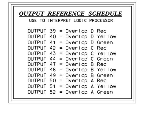
THIS ELECTRICAL DETAIL IS FOR THE SIGNAL DESIGN: 07-0766 DESIGNED: December 2014 SEALED: 3/6/2015 REVISED: N/A
