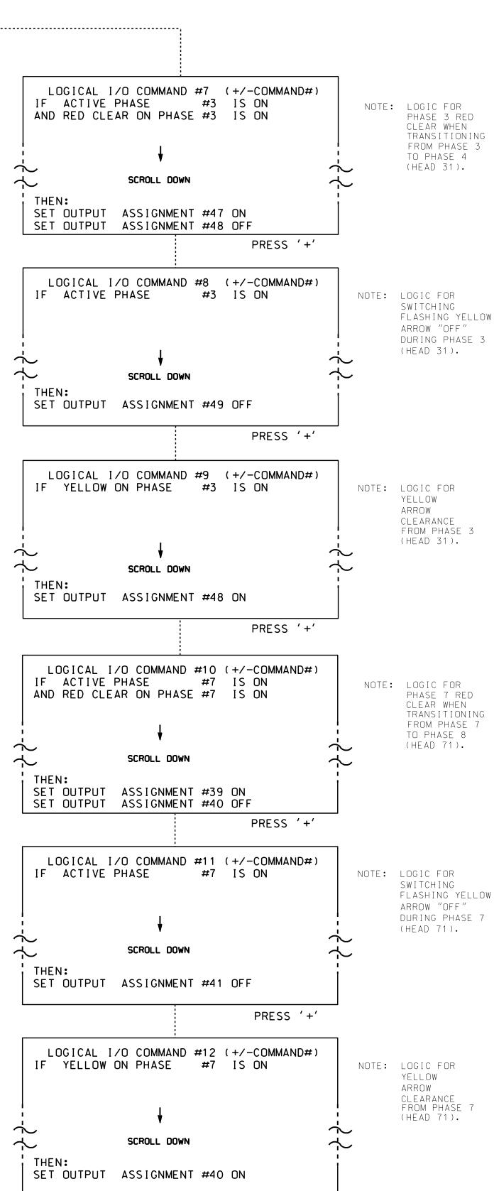
LOGIC I/O PROCESSOR PROGRAMMING COMPLETE
