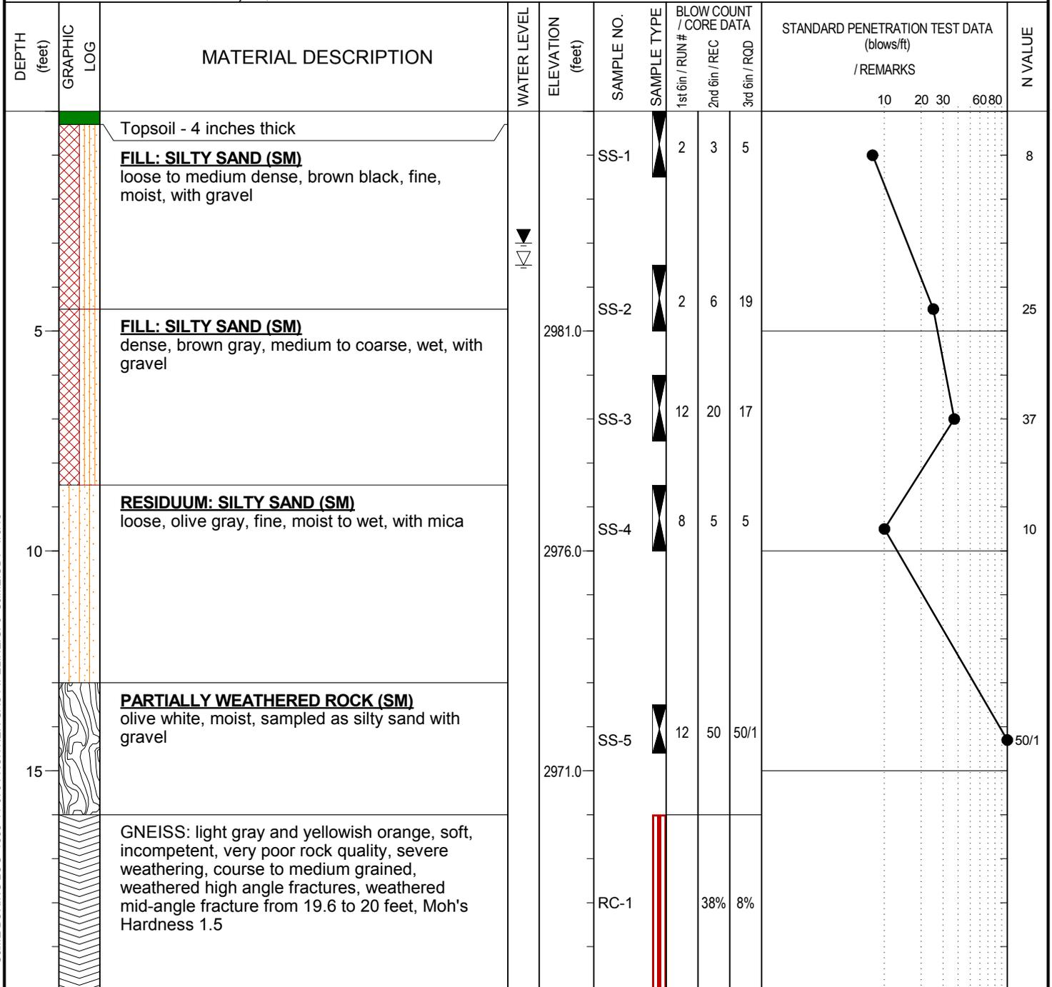
S&ME BORING LOG - 1358-14-070 FRONTIER GAS PIPELINE.GPJ S&ME.GDT 1/6/15
