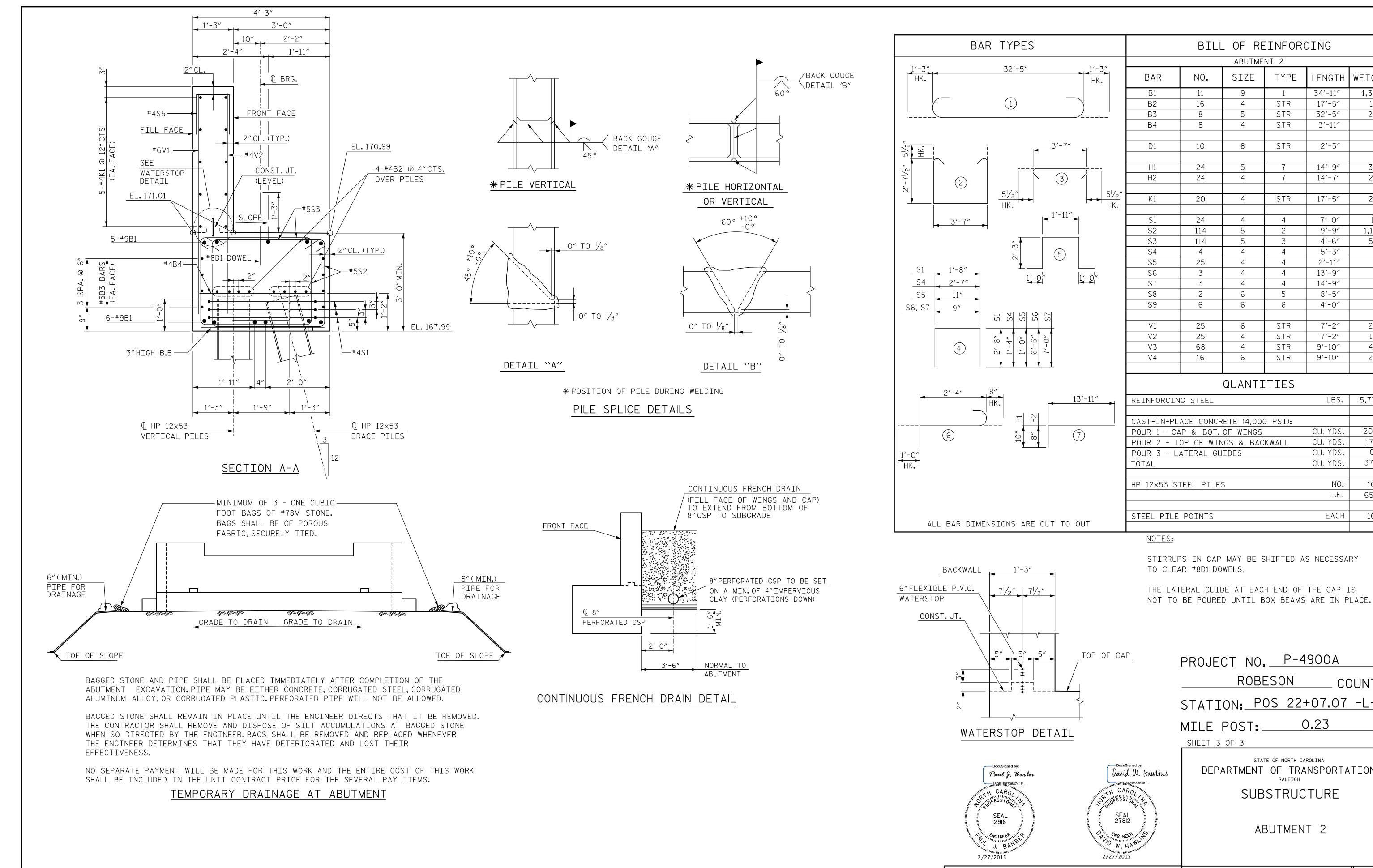
STATION: POS 22+07.07 -L-MILE POST: 0.23 SHEET 3 OF 3 STATE OF NORTH CAROLINA DEPARTMENT OF TRANSPORTATION SUBSTRUCTURE ABUTMENT 2 REVISIONS SHEET NO. S-17 NO. BY: DATE: DATE: BY: 343 E. Six Forks Rd., Suite 200, Raleigh, N.C. 27609 TOTAL SHEETS **54** DWG. NO. 17
