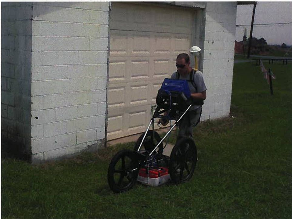
GSSI SIR-3000 Ground-Penetrating Radar with 400 MHz Antenna
